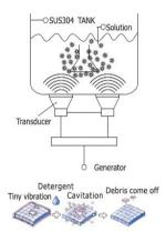
Ultrasonic cleaning is on based on the cavitation effect caused by high-frequency ultrasonic wave vibration signal in the fluid. Microscopic bubbles are formed, and they implode violently causing the cavitation which creates an intense scrubbing action on the surface of the item being cleaned. The bubbles are small enough to penetrate microscopic crevices, cleaning them thoroughly and consistently.
